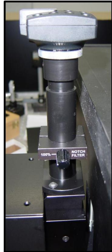
*Fig. 12 : camera viewer and rotatable notch filter knob*
